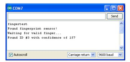
The 'confidence' is a score number (from 0 to 255) that indicates how good of a match the print is, higher is better. Note that if it matches at all, that means the sensor is pretty confident so you don't have to pay attention to the confidence number unless it makes sense for high security applications.
